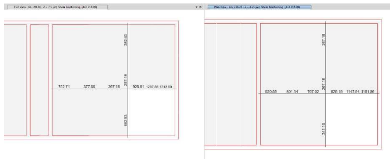
Figure 6-14 Shear Reinforcing Detail (mm 2 /m)
