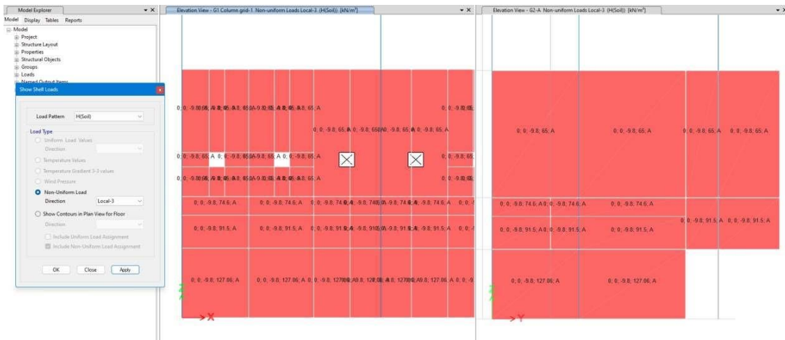
Figure 6-37 Applied Soil Load on RCC Wall
