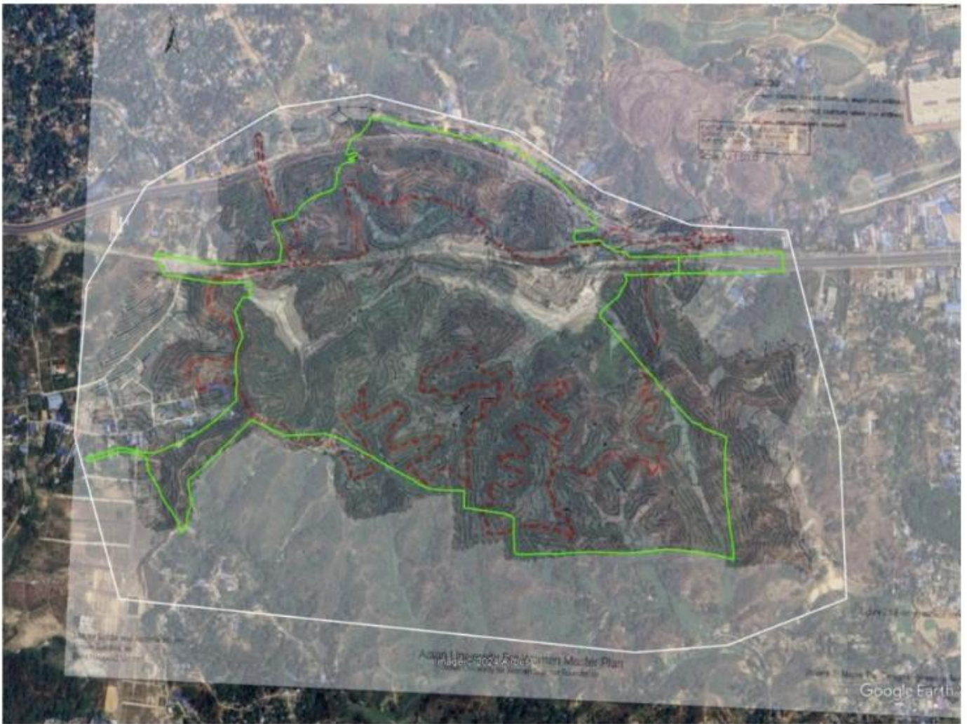
Contour map overlain on 2024 Google Earth image with proposed survey area shown in white [UAW_UAV_Survey_AOI-1.kml]. AUW site boundary shown in green.
